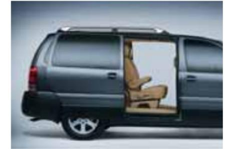
**Power sliding doors.** Opening and closing the RELAY's side doors is even easier when you can do it with the push of a button.
